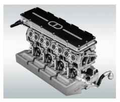
Intelligent Valve Actuation (IVA) from Camcon Auto brings real-time digital control to the gas exchange process in combustion engines. Dramatically reducing emissions and improving drivability, IVA is designed for manufacture and affordability.
