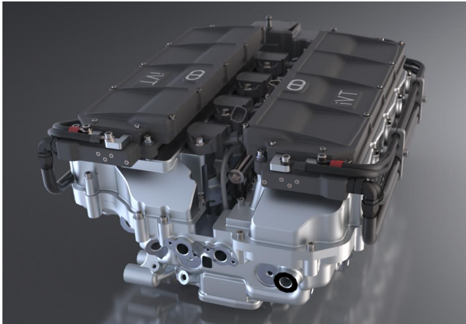
Figure 12: 16 valve, 4 cylinder in-line iVT package – based on the Jaguar Land Rover Ingenium engine
